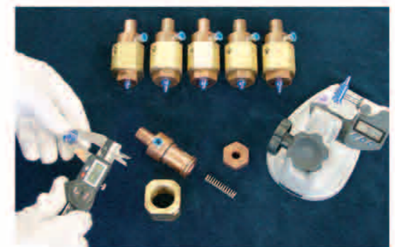
QA during the process and 100% inspection
